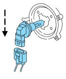
12. After the new bulb is installed, carefully let the bulb socket dangle downward near the lamp housing (Passenger side only).
